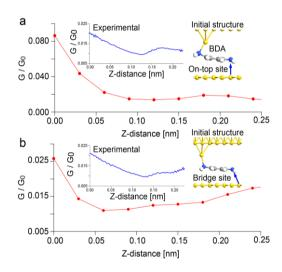
Fig. 1 Conductance curves of BDA for (a) on-top and (b) bridge sites, respectively.
